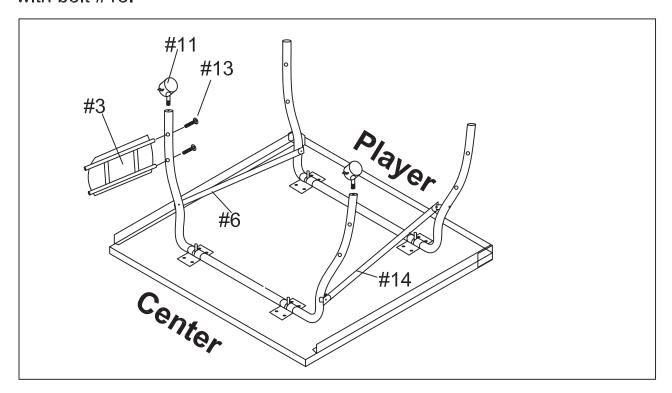
5. Turn the two table surfaces over carefully, attach the plastic plate with steel frame #3 with bolt #13 to opposite table leg as shown.
