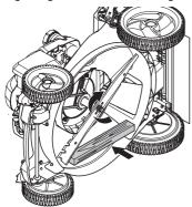
5 The bolt should be tightened with a torque of 35-40 ft. lbs. / 47-54 Nm.
