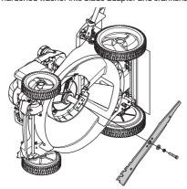
4 Use block of wood between blade and lawn mower housing and tighten the blade bolt, turning clockwise.
