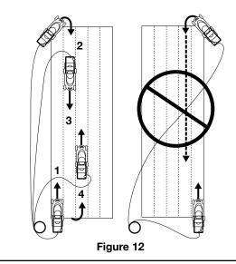
2. Place the bulk of the extension cord on the lawn close to the starting point.
