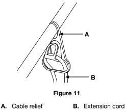
**Note:** Use a waterproof electrical extension cord rated 14AWG. H05VV-F and H05RN-F in US.
