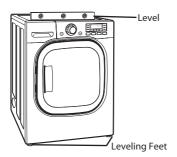
All four leveling feet must rest solidly on the floor.
