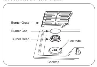
A CAUTION: DO NOT remove any parts from the cooktop until they have completely cooled and are safe to handle. Do not operate the surface burners unless all burner parts and grates are properly placed.
