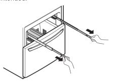
Grasp the drawer on each side and hook the door supports (1) into the rail tabs (2) located on both sides.
