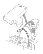
5 Hold the water supply connection and gently push in the collet to connect the water supply line as shown in 1. Insert the tube at least 5/8 inch (15 mm) into the connector.
