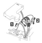
4 Rotate the hinge lever counterclockwise
