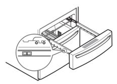
4 Reconnect the wire harness to the connection at the end of the right rail by aligning the two ends and pushing them together until you hear a click. The tabs should snap back into place. Tug gently to make sure the connection is secure.
