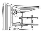
2 To remove the in-door ice bin, grip the front handle, slightly lift the lower part, and slowly pull out the bin as shown.
