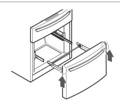
7 Using both hands, slide the two rails in simultaneously.
