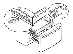
3 Remove the middle drawer by pulling the drawer out to full extension. Lift the front of the drawer up, then pull it straight out.
