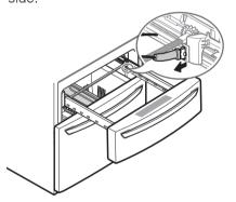
3 Remove the screws on both the left and right rails.
