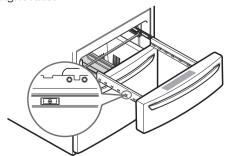
4 Grasp the drawer on each side and pull it up to separate it from the rails.
