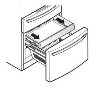
On the left rail, use a flat blade screwdriver to push in on the tab to release the drawer from the rail, as shown below. Once the left side is loose, push the tab on the right side with your finger to release the drawer. Lift the front of the drawer up, then pull it straight out.
