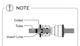
1) Gently insert the tube until only one line shows on the tube.
