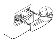
3 Lower the door into its final position and tighten the screws located on both sides.
