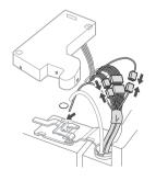
4 Push the water supply tube into the hole on the top case and pull it through the backplate.
