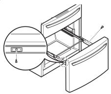
4 Insert the the top pullout drawer into the frame, and push the drawer back into place until you hear a click.
