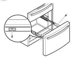
6 With both hands, grip both sides of the drawer and pull it up to remove it from the rails.
