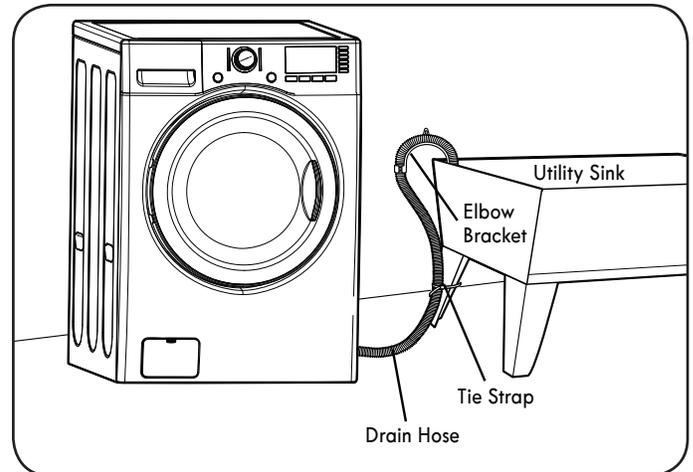
Install the elbow bracket near the end of the drain hose. Hang the end of the drain hose over the side of the utility sink. Use a tie strap to secure the drain hose in place.
