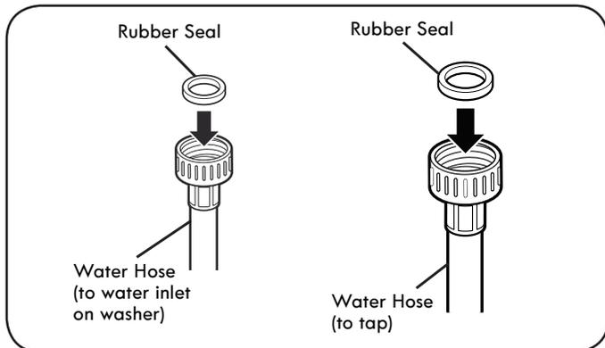
1. Inspect the threaded fitting on each hose and make sure there is a rubber seal in place in both ends.
