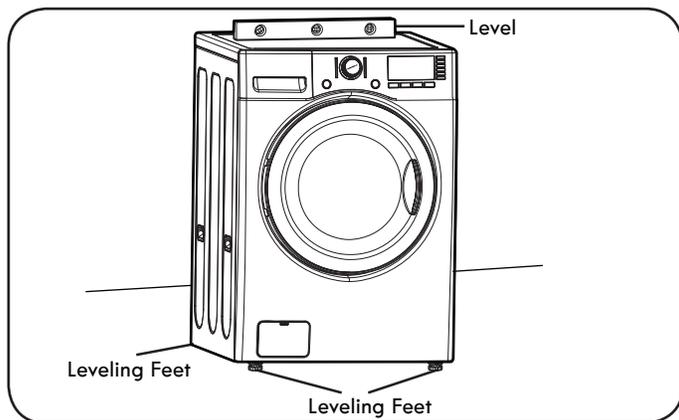
1. Position the washer in its final location, taking special care not to pinch, strain, or crush the water and drain lines. Place a level across the top of the washer.
