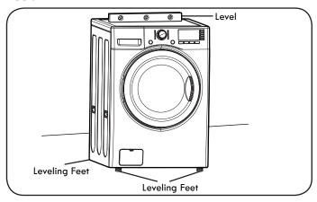
1. Position the washer in its final location, taking special care not to pinch, strain, or crush the water and drain lines. Place a level across the top of the washer.
