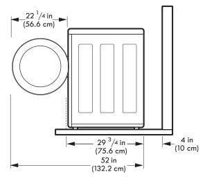
To ensure sufficient clearance for water lines and airflow, allow minimum clearances of at least 1 in. (2.5 cm) at the sides and 4 in. (10 cm) behind the unit. Be sure to allow for wall, door, or floor moldings that may increase the required clearances.
