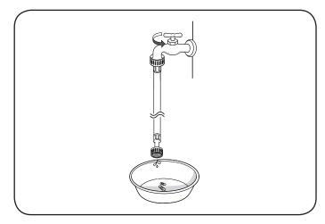
3. Always run a gallon or two (4L) of water through each inlet hose to flush dirt, scale and other debris out of the water lines. Doing so will help prevent future problems with clogged filter screens, and will also allow you to verify which hose is hot and which is cold.
