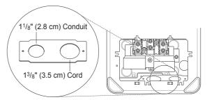
Remove the Conduit connection plate
