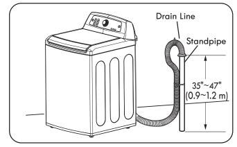
Bend the outlet end of the drain hose to form a U shape. Inset the end of the drain hose into the drain. If the drain is large enough for the flange on the hose to fit inside, then do not insert the flange more than 1-2 inches into the drain. Use the tie strap included with the installation materials in the foam block in the tub to secure the drain hose to the drain.
