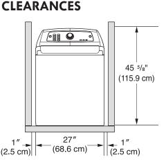
To ensure sufficient clearance for water lines and airflow, allow minimum clearances of at least 1 in. (2.5 cm) at the sides and 4 in. (10 cm) behind the unit. Be sure to allow for wall, door, or floor moldings that may increase the required clearances.
