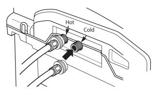
Turn OFF both water faucets completely. Unscrew the hot and cold water lines from the back of the washer.
