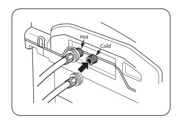
4. Attach the (red) hot water line to the hot water inlet on the back of the washer. Attach the (blue) cold water line to the cold water inlet on the back of the washer. Tighten the fittings securely. Turn ON both faucets all the way and check for leaks at both ends of the hoses.
