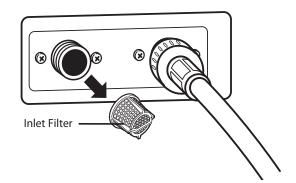
Carefully remove the filters from the water valves and soak them in white vinegar or a lime scale remover, following the manufacturer's instructions. Be careful not to damage the filters while cleaning.
