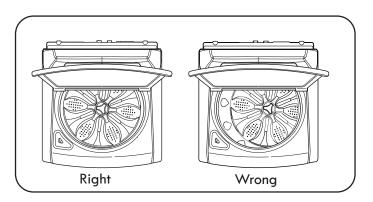
3. To make sure that the washer is properly level, open the lid and look from above to see if the tub is centered. If the tub is NOT centered (as shown in the drawing on the right), readjust the feet. If you have a level, check your washer with the level.
