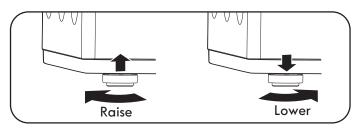
2. Adjust the leveling feet. Turn clockwise to raise the washer or counterclockwise to lower it.
