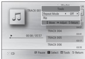
2. Press the ◀▶ buttons to select **Track, All, Shuffle, or Off**.
