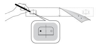
2. Mark the location where the screws will go through on the wall, and then remove the installation guide. Next, drill holes for the screws using an appropriately sized drill bit.
