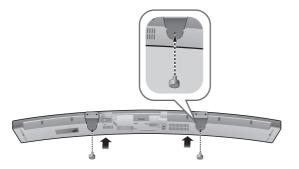
5. Insert a Holder-Fix Mount into each hole on the product's bottom side. Tighten each Holder-Fix Mount to fix the Soundbar to the 2 Bracket-Wall pieces.
