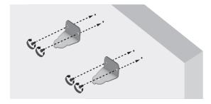
3. Fasten the 2 Bracket-Wall pieces firmly to the wall at the marked locations using the appropriate screws.
