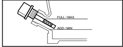
Be sure the machine is level when checking the oil level. (Refer to the engines operating manual for seasonal grades).
