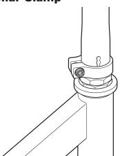
Using a 5 mm Allen wrench, check that the collar clamp bolt is tightened securely. This item is tightened and quality inspected at the factory, but there is a slight chance that the effects of shipping or handling may have caused the bolt to loosen.
