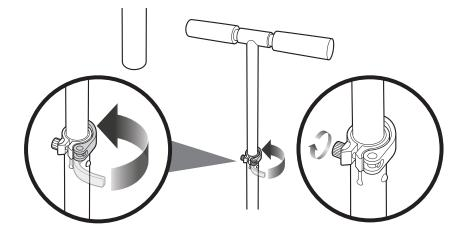
**2** The tension of the quick-release lever can be adjusted by manually tightening or loosening the Allen bolt. Be careful not to over-tighten. You should always be able to open and close the quick-release lever by hand and the T-bar should slide freely when the quick-release is open.
