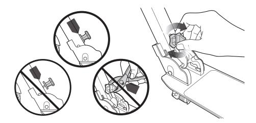
**Note:** To activate the anti-rattle feature twist the knob to the right to tighten. Please note there is no need to over tighten.
