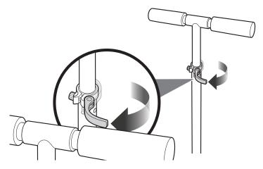
**1** To adjust the height of the handlebars, open the quick-release lever and slide the T-bar to the desired position and resecure the quick release lever to lock into place. **Note:** When the T-bar is raised to the maximum height, depress the push button located directly below the quick release lever to unlock the T-bar.
