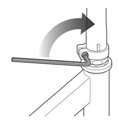
A warning: Failure to properly install and tighten the collar clamp may cause the rider to lose control and fall. If you are having difficulty understanding these instructions, please contact Razor Customer Service for assistance.
