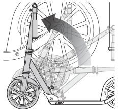
**Note:** The Anti-Rattle knob is spring-loaded and will automatically lock in the upright position when fully upright.
