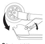
**3** To release the folding mechanism, put one foot on the deck plate and push joint release lever down. Raise handlebars up until securely locked in the upright position.
