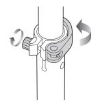
**Note:** The tension of the quick-release lever can be adjusted by manually tightening or loosening the Allen bolt. Be careful not to over-tighten. You should always be able to open and close the quick-release lever by hand and the T-bar should slide freely when the quick-release is open.
