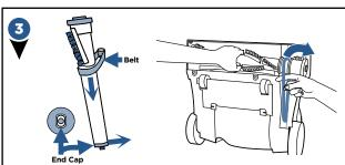
Thread belt and line up End Cap to reassemble roller. Replace bottom cover and 6 screws.
