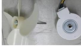
Show the left picture. If you strongly pull out the fan blade and remove, the fan and shaft of the motor will be damage and have a bad performance.
