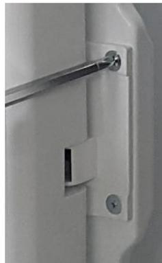
※ Assemble Procedures at Middle Hinge Part
