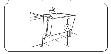
Top of tub must be at least 86cm (34 inches) high and no higher than 130cm (51 inches) from bottom of washer (A)
