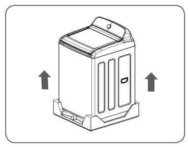
1. After removing the carton shipping material, with the aid of an assistant lift the washer off the foam base.
