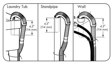
2. Secure drain hose to laundry tub leg, drain standpipe, or inlet hoses for wall standpipe with cable tie.
