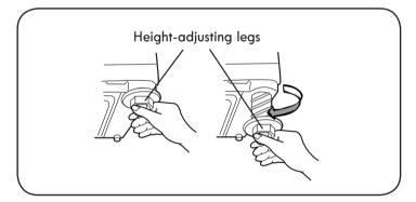
**NOTE:** You may need to use a Unit Leveler Foot if the floor is uneven on the washer back side. Place the Foot beneath washer rear leg for leveling.
