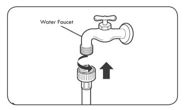
2. Connect the water supply hoses to the HOT and COLD water faucets tightly by hand and then tighten another 2/3 turn with pliers.
