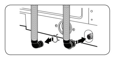
1. Attach drain hose to drain port. Squeeze clamp and slide end of drain hose onto drain port and secure with clamp.
