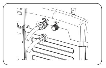
4. Attach the (red) hot water line to the hot water inlet on the back of the washer. Attach the (blue) cold water line to the cold water inlet on the back of the washer. Tighten the fittings securely. Turn ON both faucets all the way and check for leaks at both ends of the hoses.
