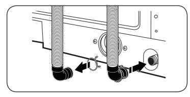
1. Attach drain hose to drain port. Squeeze clamp and slide end of drain hose onto drain port and secure with clamp.
