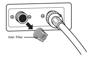
2 Carefully remove the filters from just inside the water valves and soak them in white vinegar or a lime scale remover, following the manufacturer's instructions. Be careful not to damage the filters while cleaning.
