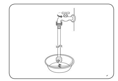
3. Always run a gallon or two of water through each inlet hose to flush dirt, scale and other debris out of the water lines. Doing so will help prevent future problems with clogged filter screens, and will also allow you to verify which hose is hot and which is cold.
