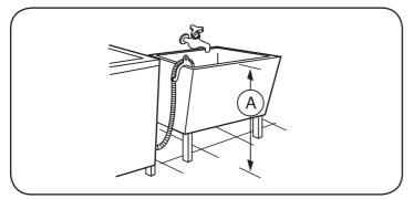
• Top of tub must be at least 34 inches (86cm) high and no higher than 51 inches (130cm) from bottom of washer (A)
