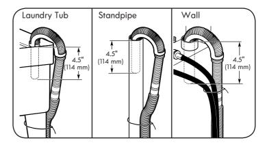
**2.** Secure drain hose to laundry tub leg, drain standpipe, or inlet hoses for wall standpipe with cable tie.
