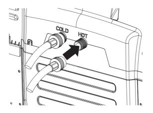
Turn OFF both water faucets completely. Unscrew the hot and cold water lines from the back of the washer.
