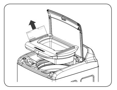
2. Save the foam block for future use. If the washer must be moved in the future, this will help prevent damage to the washer during transportation.
