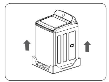
1. After removing the carton shipping material, with the aid of an assistant lift the washer off the foam base.
