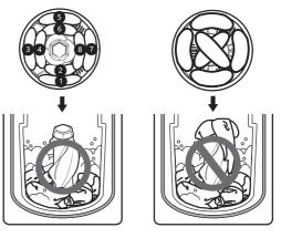
2. Load clothes loosely within the maximum guideline on the tub or surrounding the agitator. Clothes need room to circulate in order to get clean.
