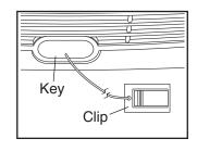
sole. After several seconds, the displays will light. IMPORTANT: In an emergency, the key can be pulled from the console, causing the walking belt to slow to a stop. Test the clip by carefully taking a few steps backward; if the key is not pulled from the console, adjust the position of the clip.
