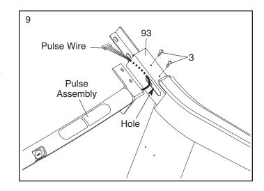
10. Slide the pulse assembly onto the Left and Right Handrails (92, 93). Make sure the brackets on the pulse assembly are flush against the rubber on the Handrails. Be careful not to pinch the pulse wire against the pulse assembly.
