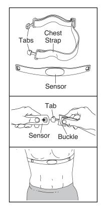
attach the other end of the chest strap to the sensor. Adjust the length of the chest strap, if necessary.
