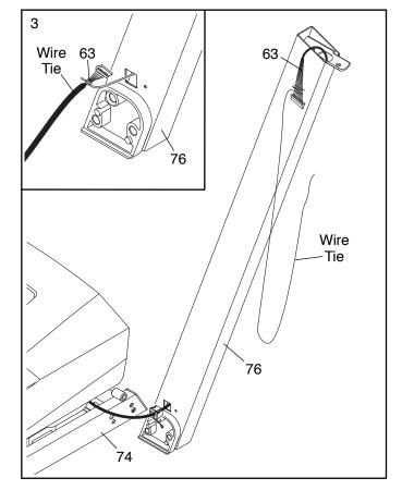
4. Lay the Right Upright (76) near the Base (74) as shown. Attach the ground wire to the Base with a #8 x 1/2" Ground Screw (1).
