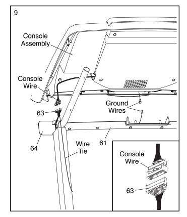
10. Insert the wires into the Right Handrail (64) through the indicated hole as you set the console assembly on the Left and Right Uprights (66, 76). **Make sure that no wires are pinched.**
