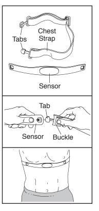
side-up. Then, attach the other end of the chest strap to the sensor. Adjust the length of the chest strap, if necessary.
