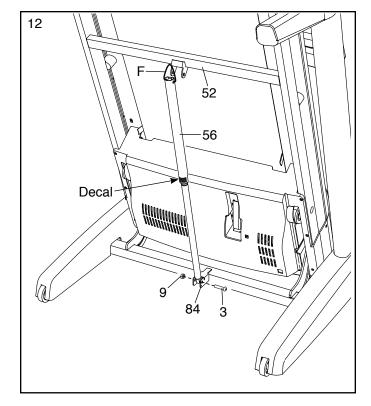
13. Align the upper end of the Storage Latch (56) with the bracket on the Frame (52). Insert a 5/16" x 2 1/4" Bolt (4) through the bracket. This should push a spacer (G) out of the other end. Discard the spacer.
