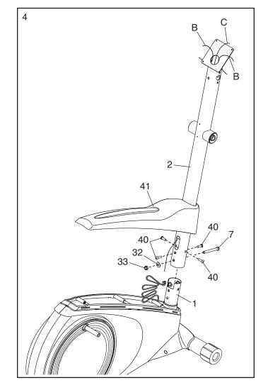
See the inset drawing. Locate the wire tie (C) in the lower end of the Upright (2). Tie the wire tie to the Wire Harness (73). Next, pull the upper end of the wire tie until the Wire Harness is routed through the Upright.
