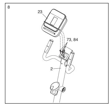
9. Insert the excess wire into the Upright (2) or into the Console (23).
