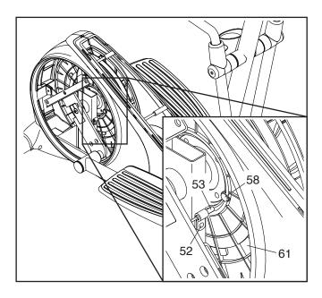
Next, rotate the Pulley (61) until a Magnet (58) is aligned with the Reed Switch (53). Slide the Reed Switch slightly toward or away from the Magnet. Then, retighten the M4 x 16mm Screw (52). Rotate the Pulley for a moment.
