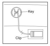
In an emergency, the key can be pulled from the console, causing the walking belt to slow to a stop. Test the clip by carefully taking a few steps backward; if the key is not pulled from the console, adjust the position of the clip.
