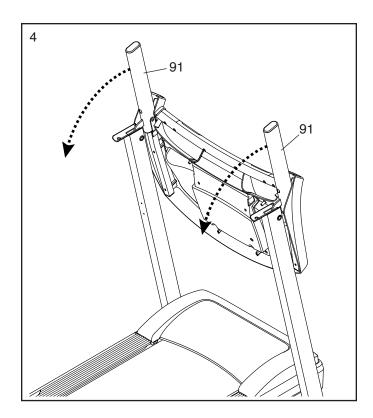
Tighten a 3/8" x 2 3/4" Screw (2) with a 3/8" Star Washer (27) into the bottom of each Handrail (91) as shown; firmly tighten the Screws.
