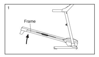
Hold the treadmill firmly with your right hand as shown. Pull the latch knob to the left and hold it. Raise the frame until the latch plate is past the latch pin. Then, slowly release the latch knob; make sure that the latch plate is resting against the latch pin.
