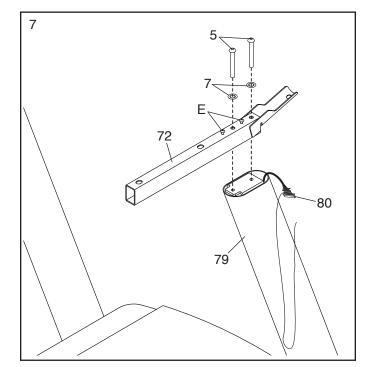
Attach the other Handrail (72) to the Left Upright (78) with two 5/16" x 2" Screws (5) and two 5/16" Star Washers (7); start both Screws, and then tighten them.
