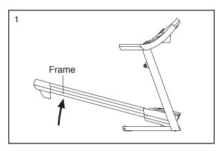
2. Hold the frame firmly with your right hand. Pull the latch knob to the left and hold it. Raise the frame until the latch plate is past the latch pin. Then, slowly release the latch knob; **make sure that the latch plate is resting against the latch pin.**
