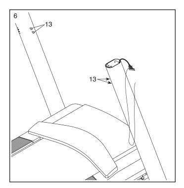
Attach a Handrail (72) to the Right Upright (79) with two 5/16" x 2" Screws (5) and two 5/16" Star Washers (7); start both Screws, and then tighten them. Make sure not to pinch the Upright Wire (80).
