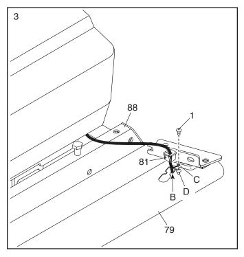
Set the Right Upright (79) on the Base (88) as shown. Make sure not to pinch the Upright Wire (80). Slide the Right Upright so that the 3/8" x 2 3/8" Screw (2) in the Base is inserted into the slot in the Right Upright. Do not tighten the Screw yet.
