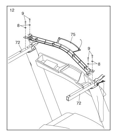
13. With the help of a second person, hold the console assembly (G) near the Handrails (72).
