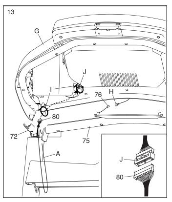
14. Set the console assembly (G) on the Handrails (72). **Make sure that no wires are pinched.**
