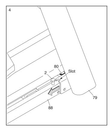
Attach the Right Upright (79) to the Base (88) with a 3/8" x 2 3/8" Screw (2), a 3/8" x 1 1/4" Screw (3), a 3/8" x 1 1/2" Screw (4), and three 3/8" Star Washers (6) as shown; do not fully tighten the Screws yet.
