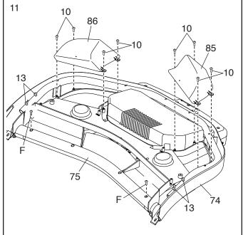
12. IMPORTANT: To avoid damaging the Pulse Crossbar (75), do not use power tools and do not overtighten the #10 x 3/4" Screws (9).
