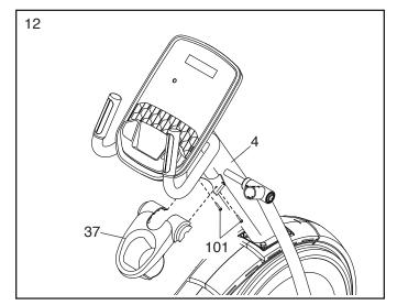
Orient a Lower Tray Cover (81) as shown, and attach it to the right side of the Accessory Tray (37) with two M4 x 16mm Screws (101).
