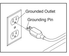
The outlet must be on a nominal 120-volt circuit.
