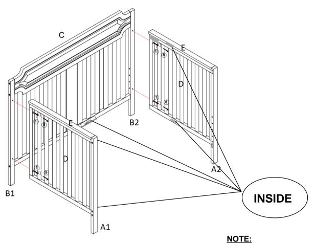
The headboard (C), side panels (D), and top rails (E), are labeled "INSIDE". To ensure proper assembly, please make sure all these parts are attached so that the INSIDE label faces inside the crib.
