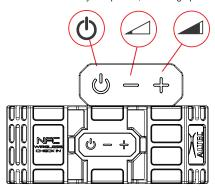
5.To power on your speaker, press and hold the " $\circlearrowleft$ " ON/OFF button for about 2 seconds.
