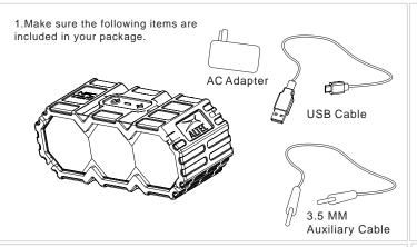
2.Connect the included USB Cable to the the included AC adapter to charge your speaker's internal battery. A full charge takes approximately 4 hours.
