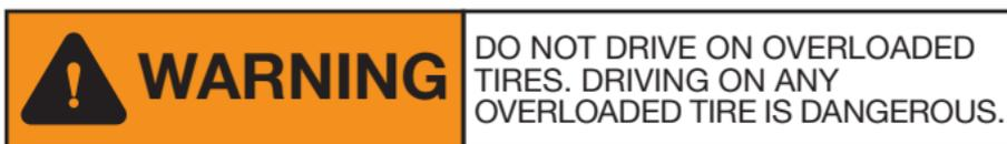
The maximum load rating of your tires is molded on the tire sidewall. Do not exceed this rating. Follow the loading instructions of the manufacturer of your vehicle to ensure that your tires are not overloaded.
