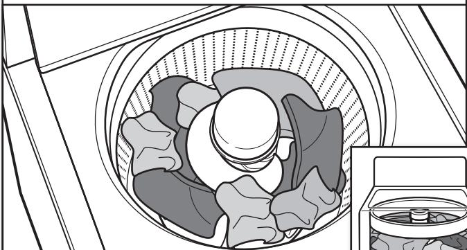
Load garments in loose heaps evenly around basket wall. For best results, do not pack the load tightly. Do not wrap large items such as sheets around the agitator; load them in loose piles around the sides of the basket. Try mixing different sized items to reduce tangling.
