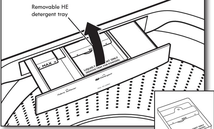
Add a measured amount of HE liquid detergent into detergent tray. This tray holds 3 oz. (89 mL). If adding powder HE detergent, remove inside tray. Do not overfill tray – adding too much detergent may cause detergent to be dispensed into the washer too early.
