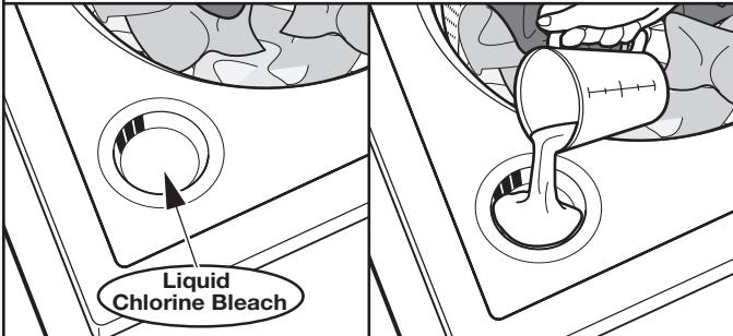
Do not overfill, dilute, or use more than 1 cup (236 mL). Do not use color-safe bleach or Oxi products in the same cycle with liquid chlorine bleach.
