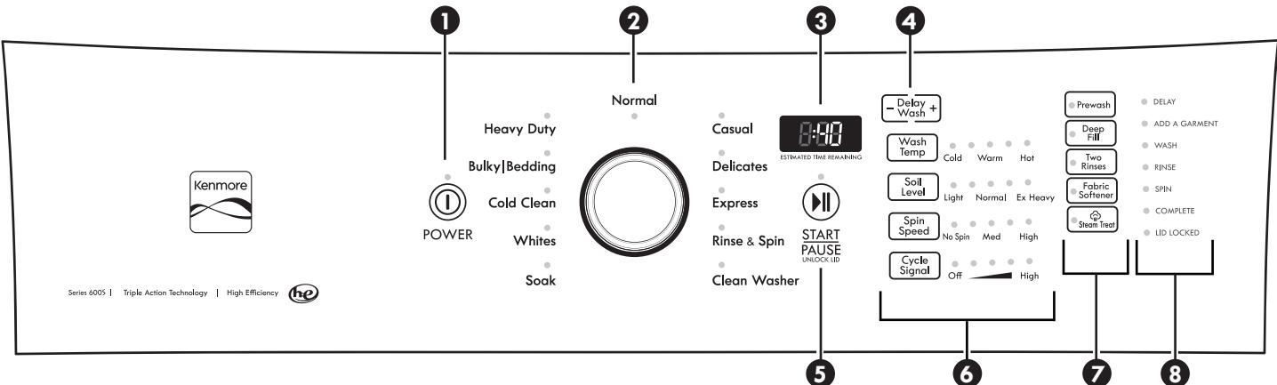
**NOTE:** The control panel features a sensitive surface that responds to a light touch of your finger. To ensure your selections are registered, touch the control panel with your fingertip, not your fingernail. When selecting a setting or option, simply touch its name until the desired section is illuminated.
