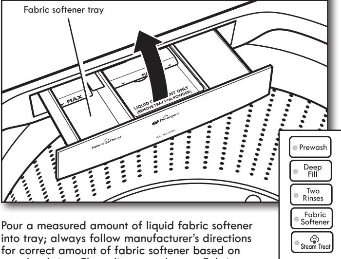
Pour a measured amount of liquid fabric softener into tray; always follow manufacturer's directions for correct amount of fabric softener based on your load size. Close dispenser drawer. Fabric softener is added during rinse.
