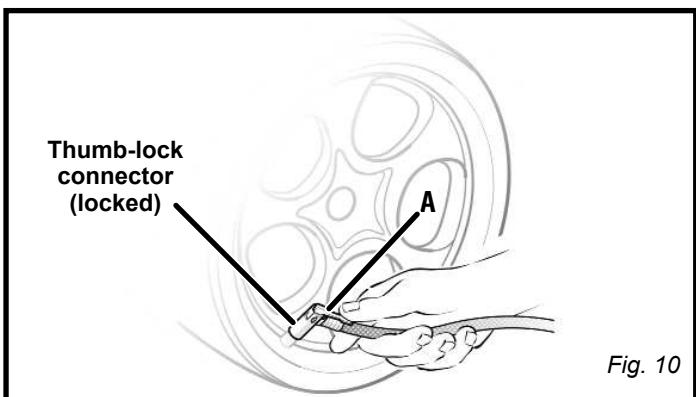
Thumb-lock connector (locked)
