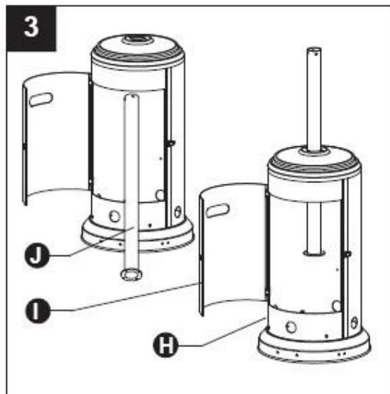
4. Secure post (J) to cylinder housing (H) using the reinforced ring (NN), M6 x 10 mm bolts (DD) and  $\Phi 6$  small flat washers (EE). Fasten and cover with the deck ring (OO).
