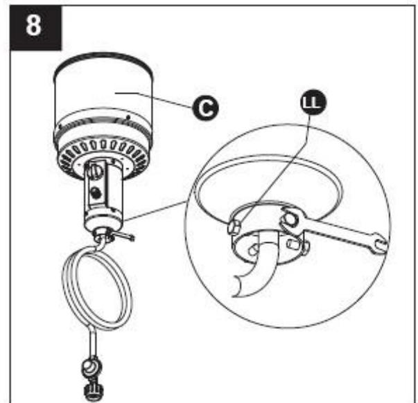
9. Insert hose of head assembly (C) into post (J). Secure head assembly (C) to post (J) with stainless steel bolts (LL).
