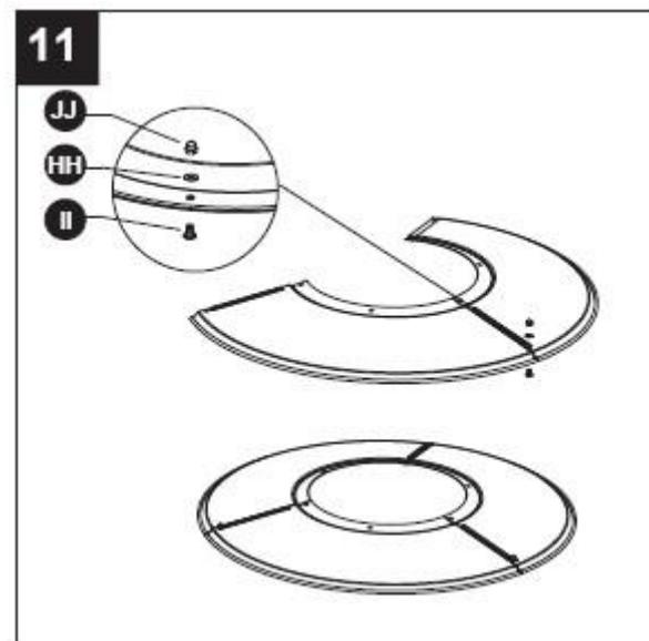
12. Attach reflector plate (B) to reflector panels (A) using M6 x 10 mm screws (II) and  $\Phi 6$  washers (HH). Secure loosely with cap nuts (JJ). Once properly aligned, tighten all screws and the preassembled bolts.
