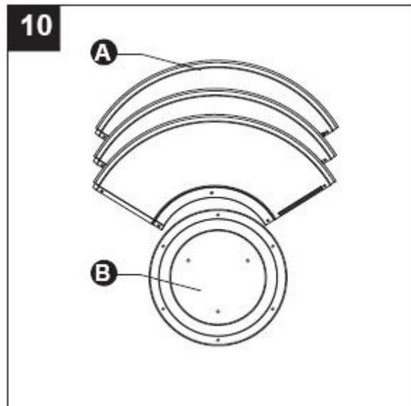
11. Attach reflector panels (A) together using M6 x 10 mm screws (II) and  $\Phi 6$  washers (HH). Secure loosely with cap nuts (JJ).
