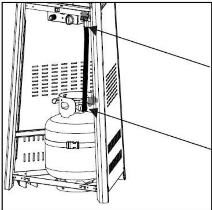
1. Make 2-3 oz. of leak check solution (one part liquid dishwashing detergent and three parts water).
