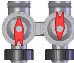
As shipped, the bypass is set-up for down-flow use. The arrow shape of the handles points in the wrong direction for UP-flow use. To convert it to UP-flow use, pull up on the red handles until they come off. Rotate the handle 180° and put it back on the valve stem.
