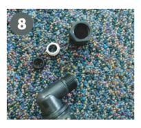
Remove the nut and sleeve from the top of the float assembly.
