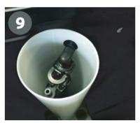
Put float assembly into the float tube.
