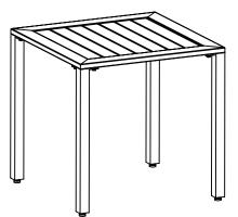
Turn over the side table, securely tighten all bolts by using Allen wrench (Gd) in a diagonal pattern. Adjust the table level by twisting knobs on the bottoms of the legs. Now your seating set is ready for use!
