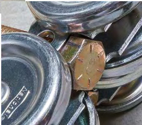
\frac{1}{2} " Bolts shown installed in Roller Assemblies
