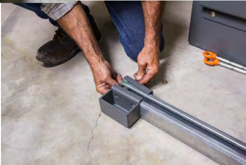
\frac{1}{2} " Bolts shown installed in Roller Assemblies
