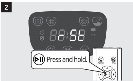
2. When "rSt" appears in the display window, press and hold the play button on the remote control.
