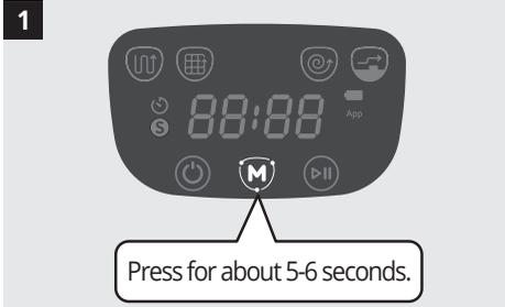
1. Press and hold the M (Mode) button on the robot display window for about 5 to 6 seconds.
