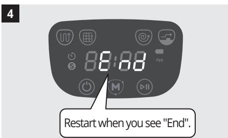
4. When "End" appears with a beep sound, turn the power off before turning it back on again.
