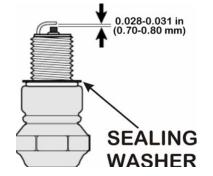
5) Install the spark plug carefu by hand to avoid cross threadi
