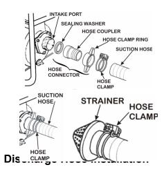
It is best to use a short, large diameter hose. This will reduce fluid friction and improve pump output. A long or small diameter hose will increase fluid friction and reduce pump output.
