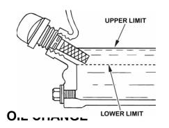
Drain the oil while the engine is warm because it will drain quickly and completely.
