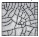
The spider-web pattern of cracking is different from a break in the aspect that it cannot be felt on the surface, unless using a fingernail; however, it does become more visually apparent when the surface is dusty or magnified. While these may appear as imperfections, crazing does not
