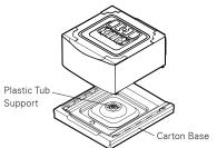
If you must lay the washer down to remove the base packaging materials, always protect the side of the washer and lay it carefully on its side. DO NOT lay the washer on its front or back.
