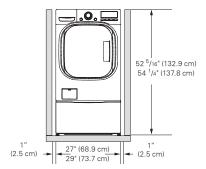
To ensure sufficient clearance for water lines and airflow, allow minimum clearances of at least 1 in. (2.5 cm) at the sides and 4 in. (10 cm) behind the unit. Be sure to allow for wall, door, or floor moldings that may increase the required clearances.
