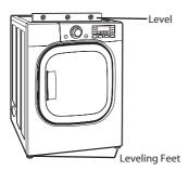
• All four leveling feet must rest solidly on the floor. Gently push on the top corners of the dryer to make sure that the dryer does not rock from corner to corner.
