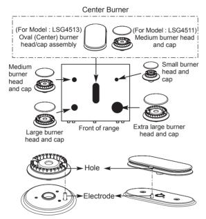
Make sure the hole in the burner head is positioned over the electrode.
