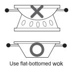
Do not use a wok support ring. Placing the ring over the burner or grate may cause the burner to work improperly, resulting in carbon monoxide levels above allowable standards. This can be
