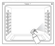
5 Spray or pour the remaining water onto the bottom center of the oven cavity. The indentation on the oven bottom should be fully covered to submerge all soils. Add water if necessary.
