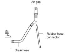
Attach the rubber connector to disposal or waste tee with the hose clamp provided. Move into position and tighten the hose clamp.
