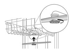
After assembly, check whether the spray arms rotate freely.
