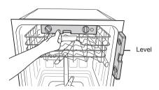
Make sure that the gap between the door and the tub is equal on both the left and right sides.
