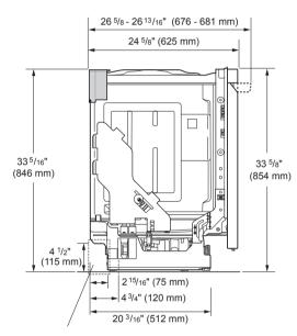
Water supply hose, drain hose and electric cable should be passed through this area.
