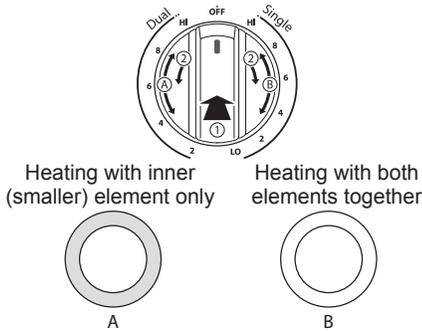
**Turning on a Triple element (on some models)**
