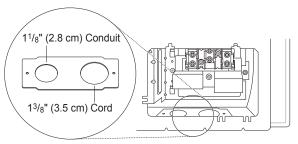
Remove the conduit connection plate
