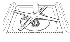
Water level should be near the center of both tub lower indentations.
