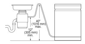
If the end of the drain hose does not fit the drain line, use a heat and detergent resistant adapter (not supplied). These may be obtained from a local plumbing supply store.
