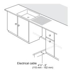
Make sure the electrical cable is oriented in the right side channel.
