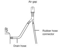
3 Attach the rubber connector to disposal or waste tee with the hose clamp provided. Move into position and tighten the hose clamp.
