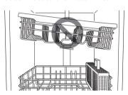
There is a 24 <sup>5</sup>/<sub>8</sub> inches (56 mm) gain in height when the upper rack is moved to the lower position.
