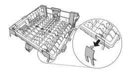
• Press the tab to remove the cable tie by hand. Cutting the tie with a knife or scissors may damage the rack or the silverware basket.
